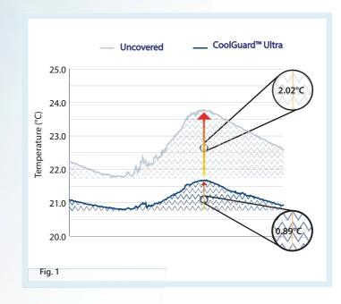
In the summer of 2022, testing was conducted on outdoor test pools, located at our state-of-the-art testing facility in South East England. The scope of these tests was to determine the benefits of covering an outdoor pool with CoolGuard™ Ultra material with GeoBubble™ technology. In order to achieve this one test pool was fitted with a CoolGuard™ Ultra cover fabricated in house, and another left uncovered to act as a control.
