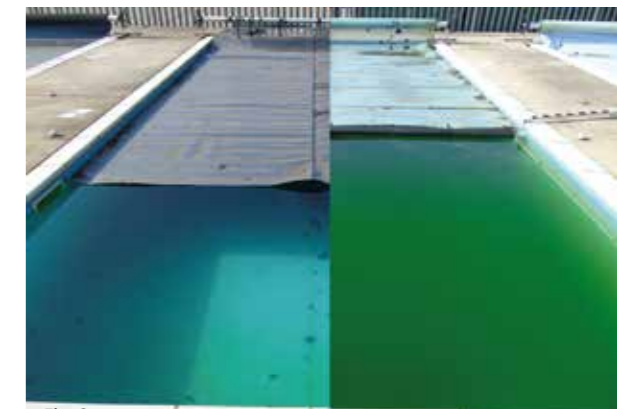
Fig. 3 The above composite image (Fig. 3) shows pools covered with EnergyGuard™ Selective Transmission (L) and a transparent cover (R) over the winter period. The pool covered with EnergyGuard™ Selective Transmission was significantly cleaner than the other pool.
